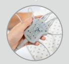
Anatomically designed cable to minimise tangling and lead reversal
